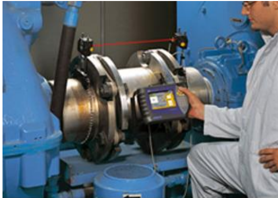
Laser shaft alignment
